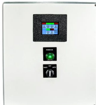
HELIPORT LIGHTING CONTROLLER PHC-61001-AC-TS With color touchscreen
